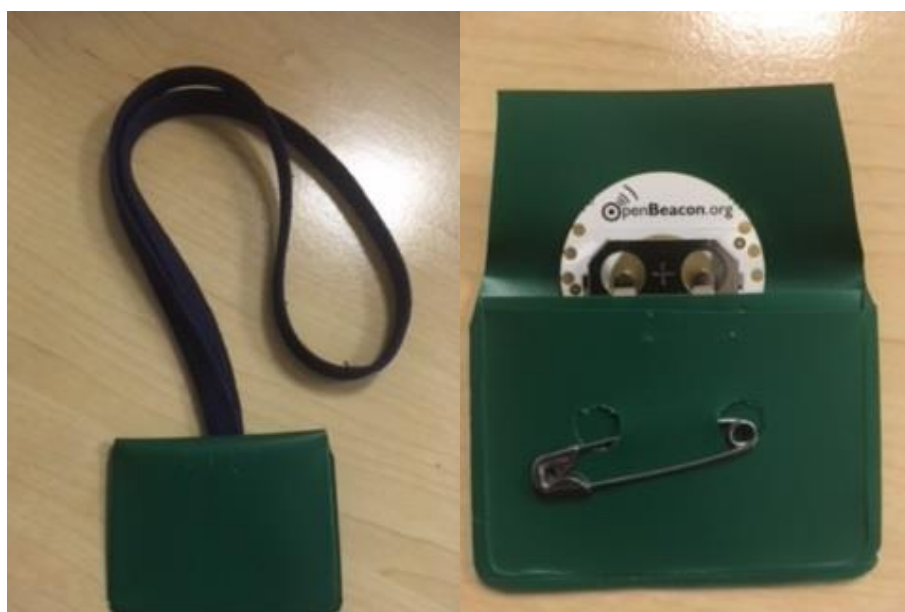
Figure 2: Packaging of proximity sensor
